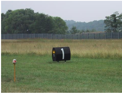
Fig. 10 Runway Distance Remaining Sign
