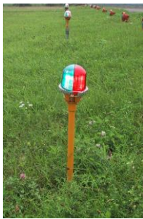
Fig. 8 Runway End/Threshold Lights
