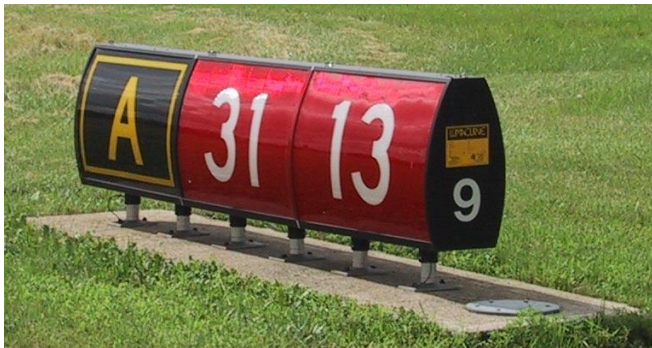
Fig. 9 Runway Holding Position Sign
