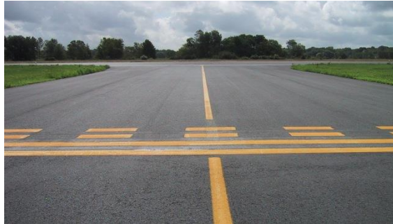
Fig. 5 Runway Holding Position Marking
